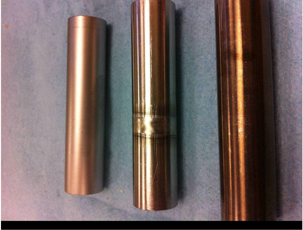
Stainless Steel Passivation by Picklex® 20 By Dipping process with Zero Waste Disposal
